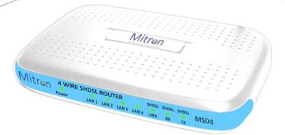
The MSD4 SHDSL router is highly suited to the specific needs of multiple users in small/home offices or remote/branch offices. The MSD4 supports high-speed symmetric data transmission, and adaptive multiple data rates. Under 4-wire operation, the MSD4 data rates can be up to 4.6 Mbps; and under 2-wire operation the MSD4 can be up to 2.3 Mbps, over an ordinary telephone line.
